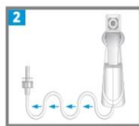
2 Hose is coiled inside sprayer. Pull out and fully extend (approx. 90cm)
